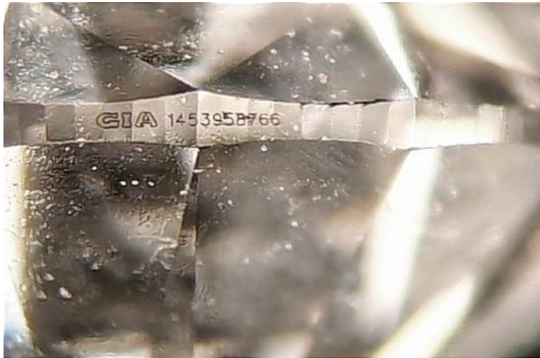
Photo 005 – Laser inscription of one of the stones examined by the Gem-Tech laboratory with a visible GIA logo that appeared to be identical to the original. (Photo: Gem-Tech)
